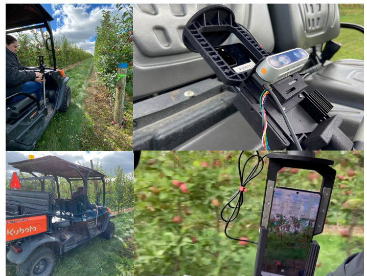
Figure 1. Scanning of an orchard using Farm Vision equipment, including cellphone, RTK GPS, and battery pack, affixed to stabilizing device (3 ft pole). This equipment will no longer be used in 2023. Harvest scans were conducted with two people using an ATV. One person drove the ATV and a cell phone operator scanned full rows (both sides) as shown in the cell phone screen. Photo: Mario Miranda Sazo.
