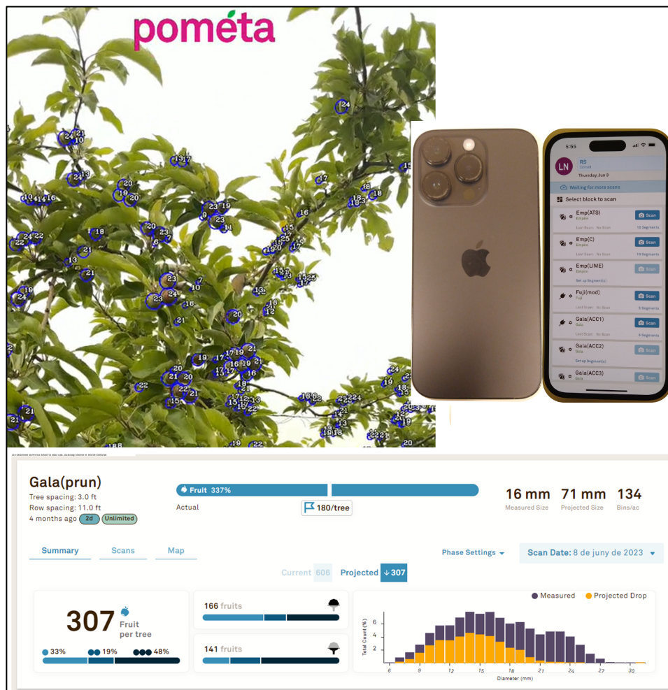
Figure 3. Fruitlets detected with the Pometa vision system and information derived from the scans in New York in 2023. Blue dots on the tree in the photograph indicate detected fruitlets. The dashboard shows the details of each scan, including number of fruitlets detected, fruit size, and the adjusted number of fruitlets expected to persist (purple bars in graph) or abscise (yellow bars).
