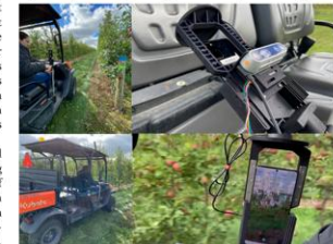
Figure 1. Scanning an orchard using Farm Vision equipment, including cellphone, RTK GPS, and battery pack, affixed to stabilizing device (3 ft pole). This equipment will no longer be used in 2023. Harvest scans were conducted with two people using an ATV. One person drove the ATV and a cell phone operator scanned full rows (both sides) as shown in the cell phone screen. Photo: Mario Miranda Sazo.
